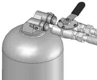
Return the tank to the service location. Install the bypass valve onto the tank head. Install and tighten the retaining clips.
