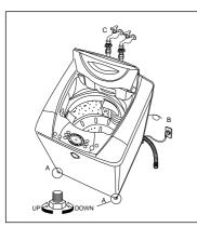
If the washer is installed on an unsuitable floor, it could make considerable noise, vibration and cause a malfunction. If washer is not level, adjust the front leg(A) up or down for horizontal setting.
