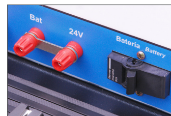
Jumper / Battery Switch
