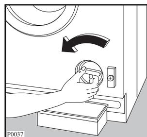
Unscrew and remove the filter.
