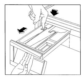
To facilitate cleaning, the upper part of the fabric softener compartment can be removed.
