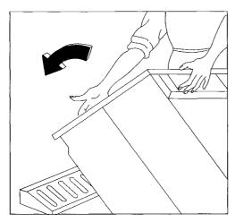
Remove the polystyrene panel from underneath the machine.
