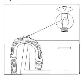
Over the edge of a basin: in this case you must ensure that the hose cannot move when the water is drained. Secure it to the wall with a hook, for example, or to the tap by means of a piece of string.
