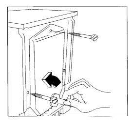
Remove the three plastic pins from the holes where the screws were previously fitted.
