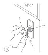
If the door has to be opened from left to right, invert the position of the plates (7), the magnet (4) and the plate (5) (Fig. B and E). Mount the countermagnet (6) and the hinges (1) as previously described.
