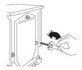
Remove the polystyrene base and take off the bottom panel by unscrewing the central screw.
