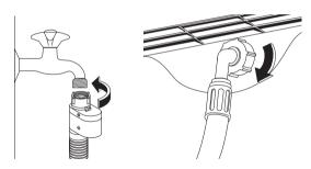
the fitting, rotate the hose and retighten the fitting, making sure there are no water leaks.
