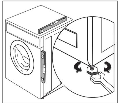
The machine must not be installed in rooms where the temperature can drop below 0°C. The water inlet hose and the drain hose must not be kinked. Please ensure that when the appliance is installed, it is easily accessible for the engineer in the event of a breakdown. Carefully level by screwing the adjustable feet in or out. Never place cardboard, wood or similar materials under the machine to compensate for any unevenness in the floor.
