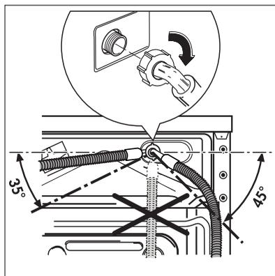
3. Set the hose correctly by loosening the ring nut. After positioning the inlet hose, be sure to tighten the ring nut again to prevent leaks.
