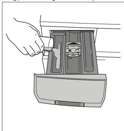
2. If required, pour fabric softener into the compartment marked
