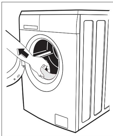
6. Fill the smaller upper hole and the two large ones with the corresponding plastic plug caps supplied in the bag containing the instruction booklet.
