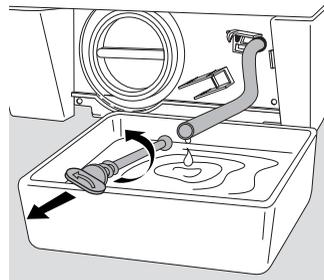
Discard the water from the container, replace it under the emergency emptying hose and remove the plug from the hose.
