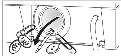
5. Check whether the pump wheel right at the back of the pump housing can turn. (If the wheel rotates with a jerky motion, this is normal.) If the pumping wheel cannot be turned, please contact your local Service Force Centre.
