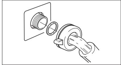
**Important!** Do not position the inlet hose vertically downwards. Position it to the right or the left as shown in the illustration.
