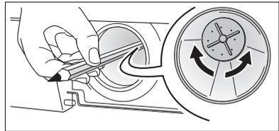
6. Insert the pump cover. Insert the guides at the sides of the cover into the guide slots and tighten the cover by turning in a clockwise direction.
