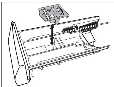
5. Clean the entire drawer recess area of the washing machine, in particular the jets on the upper side of the washing-in chamber, with a brush.
