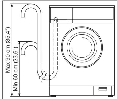
The upright standpipe should have a minimum length of 30 cm (12") from the bottom of the elbow to the top of the pipe (see diagram). Make sure that it is designed in such a way that the end of the drain hose cannot be covered with water.
