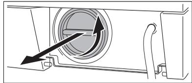
4. Remove foreign bodies and fluff from the pump housing and from the pump wheel.
