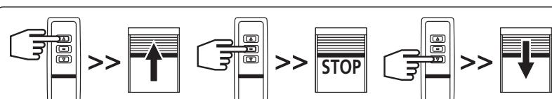
**[P0] - [04] : 3-button mode:** This mode is used to set separate controls for opening, closing, and stopping the door.
