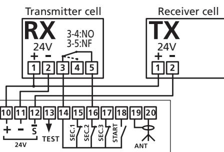
Wiring of sequential control switches
