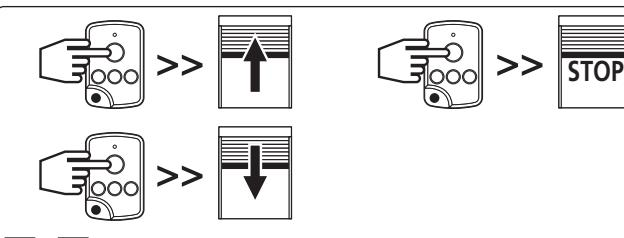
**[P0] - [02] : Sequential mode:** Cyclic operation (up / stop / down / stop...). Pressing during opening or closing stops without reversion.
