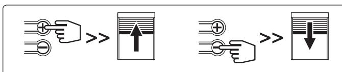
**[P0] - [05] : Forced mode with the **⊕** and **⊖** keys on the keyboard (default mode):** This mode is used to control the door using the **⊕** and **⊖** keys on the RSA Hz box in the endstop adjustment phase.
