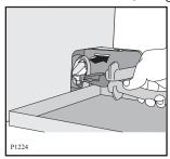
when no more water comes out, unscrew the pump cover, using a pliers, and remove the filter.
