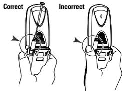
**Important:** To maximize performance when using your phone, extend the antenna before a call and do not touch the antenna during a call.
