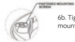
6b. Tighten down the mounting screws.
