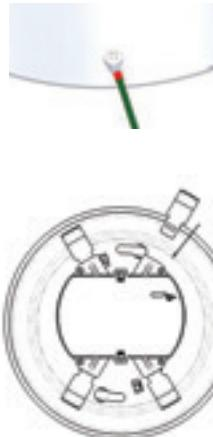
3. Snap the mounting springs into place as shown. You should not be able to remove mounting springs once installed.
