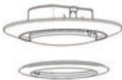
3. Partially fasten the flat head mounting screws into the j-box. Two each of the following 8-32 fasteners have been provided, select fasteners as needed for the junction box.
