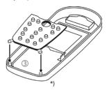
\*) If there are small pins at the bottom of the faceplate: position the tabs on both sides of the keypad mat precisely on these pins. before carrying out step ④.
