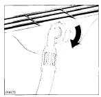
The other end of the inlet hose connected to the machine can be turned in any direction. Simply loosen the fitting, rotate the hose and retighten.
