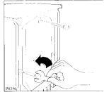
Fit the grid on the bottom of the machine and re-fit the four feet
