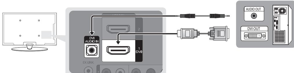
The diagram shows a television connected to a PC. On the TV's rear panel, an 'EX-LINK' port is visible. Two cables are connected: one to the 'DVI AUDIO IN' port and another to the 'AUDIO OUT' port. On the right, a PC tower is shown with 'AUDIO OUT' and 'DVI OUT' ports. The PC's 'DVI OUT' port is connected to the TV's 'DVI AUDIO IN' port. The PC's 'AUDIO OUT' port is connected to the TV's 'AUDIO OUT' port.
