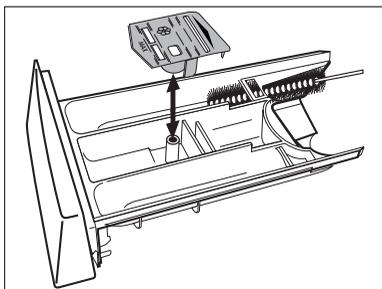
5. Clean the entire drawer recess area of the washing machine, in particular the jets on the upper side of the washing-in chamber, with a brush.
