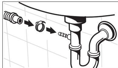
**Important!** The end of the drainage hose must not be submerged in the pumped-out water. Otherwise, the water could be sucked back into the appliance.
