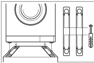
**If the appliance is to stand on a floor which moves, e.g. a suspended wooden floor:**
