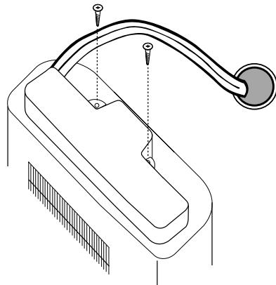
**EG** Fix the coupling cover of the outdoor unit and seal the hole in the wall around the flexible tube.
