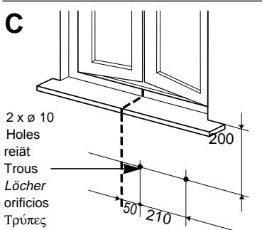
**EG** Or hanged to the wall below the window sill using the basket or the support supplied as accessory. After placing the unit in the basket check that it is levelled.
