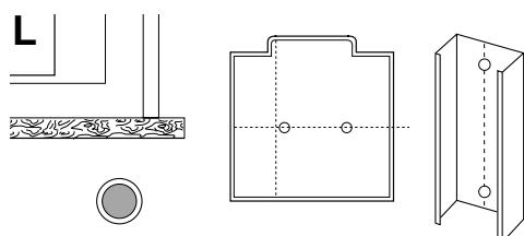
**EG** In this case: mark the holes to be drilled in the wall using the template or the support (keep levelled). Drill 2 holes 10 mm dia.
