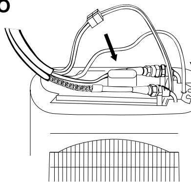
**EG** Connect the condensate plastic tube and the electric connector.
