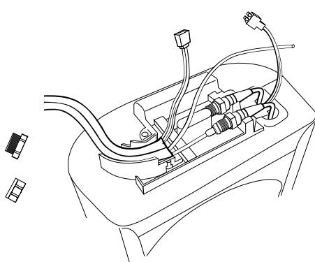
**EG** Remove the plastic plugs from quick couplings, connect the couplings by hand, then tighten using the torque wrenches (tightening torque 150 ÷ 165 Kg cm).
