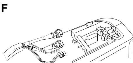
**EG** Protect quick coupling (on flexible tube and outdoor unit) with plastic plugs supplied as accessories. To insert the tubing into the hole in the wall easily and without damages, join the pipe ends and wrap them with adhesive tape.
