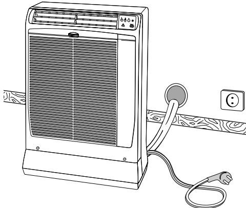
**EG** Insert the flexible tube into the hole drilled in the wall. Place the unit against the wall, if necessary, adjust the **four antivibration supports** in order to keep the unit levelled.
