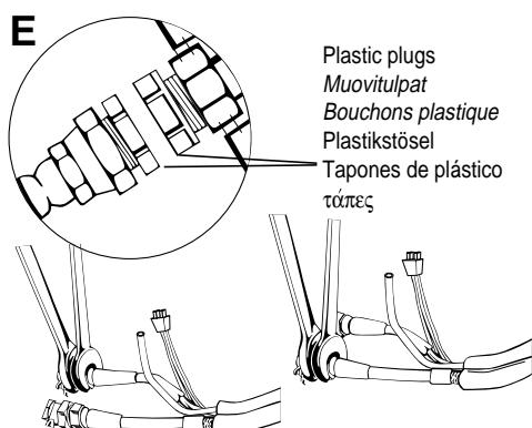
**EG** Loosen the quick coupling using the 19-21 mm spanners first and then the 19-24 mm spanners. Unscrew the flare nuts by hand and disconnect the flexible tube.
