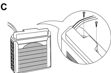
**EG** Remove the coupling cover of the outdoor unit.
