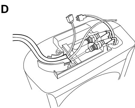
**EG** Disconnect the condensate plastic tube and the electric connector.
