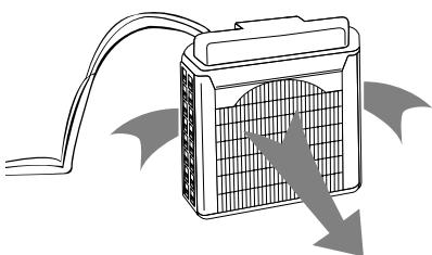
**EG** The outdoor unit may be placed on a balcony. Make sure to put it in vertical position and levelled. During the installation do not kink the connection tube between the units. Verify the correct air circulation around the outdoor
