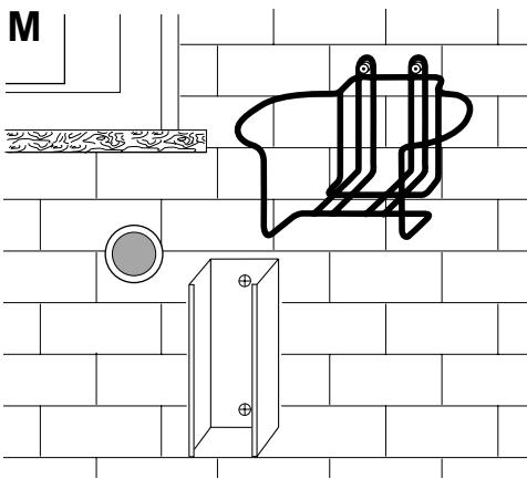
**EG** Fix the basket or the support to the wall using the expansion bolts supplied as accessory (M 6 x 20).
