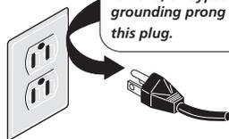
Power supply cord with 3-prong grounding plug
