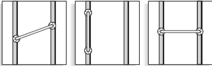
2. Precisely mark the wall for all mounting holes being used, making sure that at least TWO (2) screws in each mounting flange will securely contact a wood stud within the wall.
