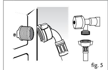
**For your washing machine to work properly, the mains water pressure must be between 0.05 and 1MPa (0.1 - 10 bar).**
