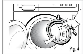
**The drain hose must be securely fastened to the outlet to prevent any risk of the drain hose becoming detached and causing flooding.**
