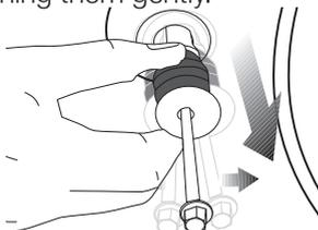
3. Fit the covers (supplied in the bag with the Operation Manual) into the holes on the rear panel. ("P")
