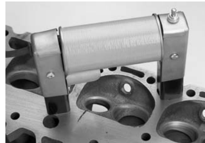
Position the magnet on the head surface. The dust will clearly show cracks between the poles of the magnet, even cracks below the surface.
