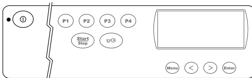
4. Press **ENTER** to save your setting and return to the Main Program screen. The LCD will display the new setting.
