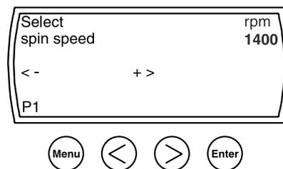
2. Use the **Arrow** buttons to raise or lower the spin speed setting. To omit the spin cycle, press the arrow button until "No Spin" displays. To omit the spin and final drain cycles, press the arrow until "No Drain" displays. (*Note:* You will have to run a drain program to open the door.)
