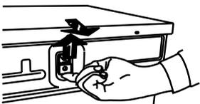
3. Rotate the spacer so that the extruded end points toward the machine.
