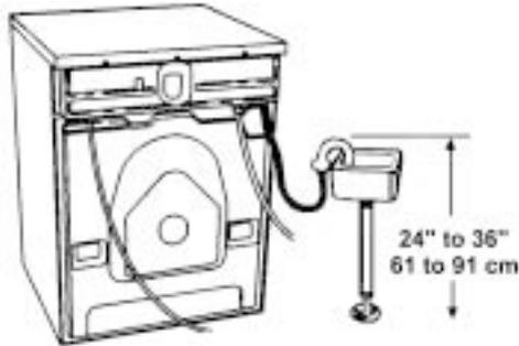
**WARNING!** Do not extend the drain hose higher than 36" (914 mm) from the bottom of the unit.
