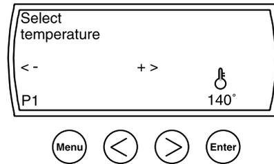
2. Use the **Arrow** buttons to raise or lower the temperature setting.
