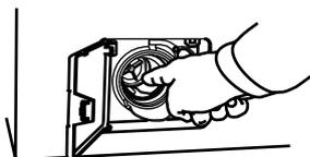
7. Replace the drain cover and reconnect the drain hose securely to its position on the door.
