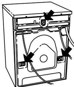
You must remove the shipping supports before you install the washer.
