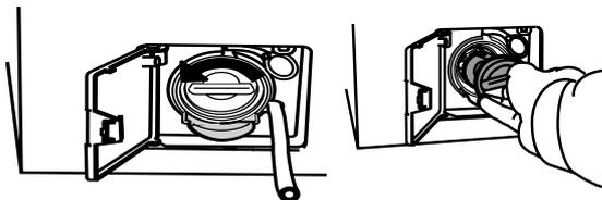
6. You can now clean out any grit or small objects. You should also clean the pump rotor at the back of the pump housing.
