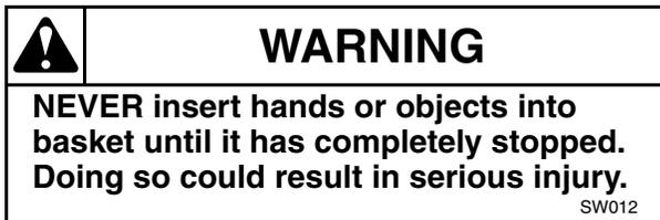
A lengthy stop procedure ensures that the basket has adequate time to stop (from the machine's highest speed) before the computer allows the door to be opened. This is an important safety feature.
