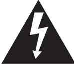
The lightning flash and arrowhead within the triangle is a warning sign indicating the presence of dangerous voltage.
