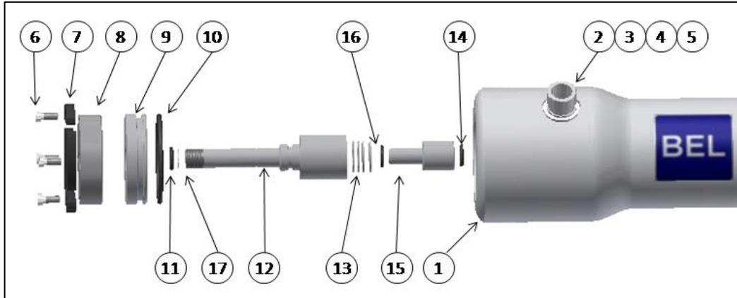
Fig 3.2 – Despiece Cabeza tubo BEL 4" 600/1000/1200 psi
