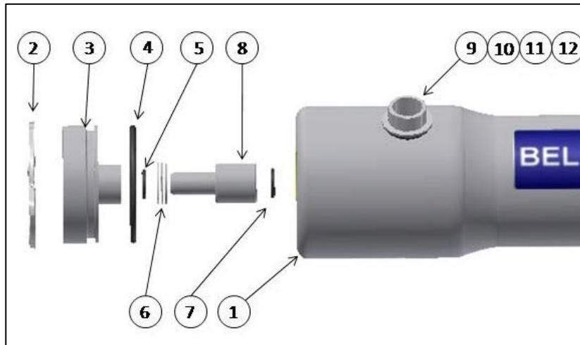
Fig 3.1 – Despiece Cabeza tubo BEL 4" 300/450 psi
