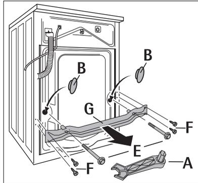
**Important!** Press all sealing caps B (2 off) and C (1 off) in firmly, so that they snap into place. (Splash protection).
