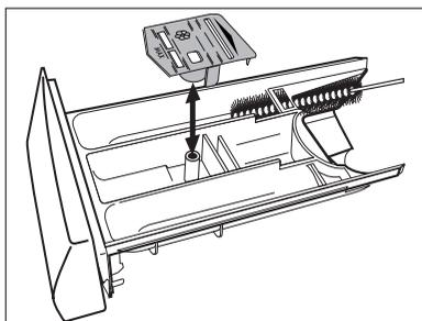
5. Clean all parts of the washing machine, especially the nozzles in the top of the washing-in chamber, with a brush.
