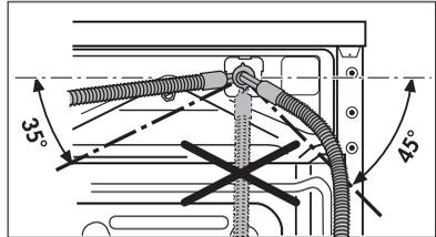
2. Connect the hose with the straight connector to a water tap with an R  $\frac{3}{4}$  (inch) screw thread.
