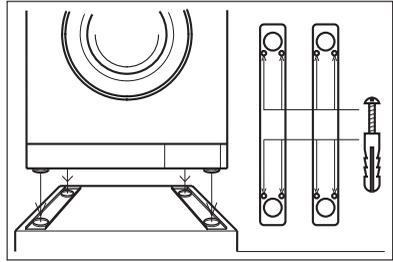
**If the appliance is to stand on floors that vibrate, e. g. floors of wooden joists with deal boards:**
