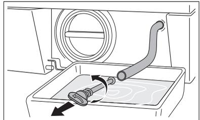
4. The water runs out. If it is necessary to empty the container more than once, seal up the emergency drain hose with the drain plug while you are doing so.
