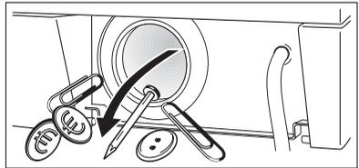
5. Check whether the pump wheel right at the back of the pump housing can turn. (It is normal for the pumping wheel to turn jerkily.) If the pumping wheel cannot be turned, please contact the Customer Care Department.
