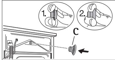
5. Seal hole using sealing cap C.
