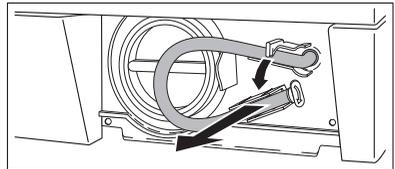
3. Place a shallow container underneath it. Then loosen the drain plug by turning it in an anti-clockwise direction and pull it out.
