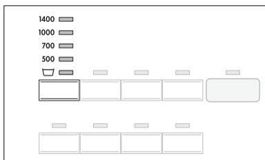
Press the spin/☒ (RINSE HOLD) button a number of times until the desired indicator lights up.
