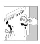
You can now see the openings that must be closed with the caches in the pack attached to the washing machine; do not forget to fold down the central capsule.
