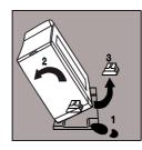
Remove all packing from the washing machine. Tilt the washing machine sideways and then remove the packing under the motor, and straighten the washing machine.
