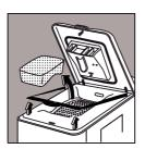
Open the washing machine lid and remove the immobilization packing and plastic films. Close the lid.
