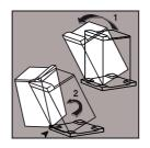
Tilt the washing machine back-wards, rotate it by a quarter of a turn on one of its corner to remove the transport base.
