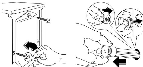
👉 Pull out the three plastic spacers from the holes into which the bolts were fitted.
