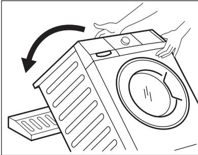
6. Put the front piece on the floor behind the appliance. Carefully put down the appliance with the rear side on it. Make sure not to damage the hoses.
