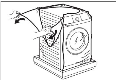
4. Remove the internal film.
