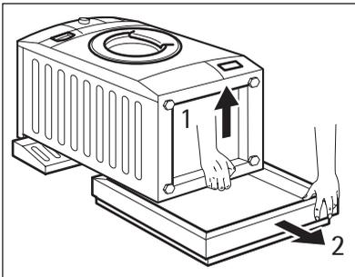
7. Remove the polystyrene protection from the bottom.
