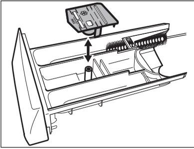
3. Remove the top part of the liquid additive compartment.
