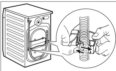
9. Remove the power supply cable and the drain hose from the hose holders.
