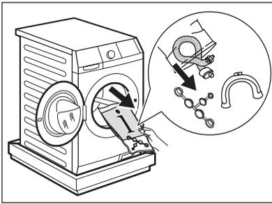
5. Open the door. Remove the polystyrene piece from the door seal and all the items from the drum.
