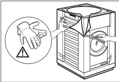
1. Use the gloves. Remove the external film. If necessary, use a cutter.
