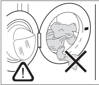
Make sure that no laundry stays between the seal and the door. There is a risk of water leakage or damage to the laundry.
