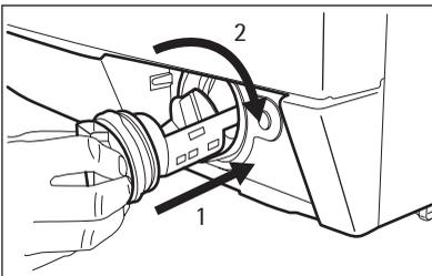
3. Put a container below the recess of the drain pump to collect the water that flows out.
