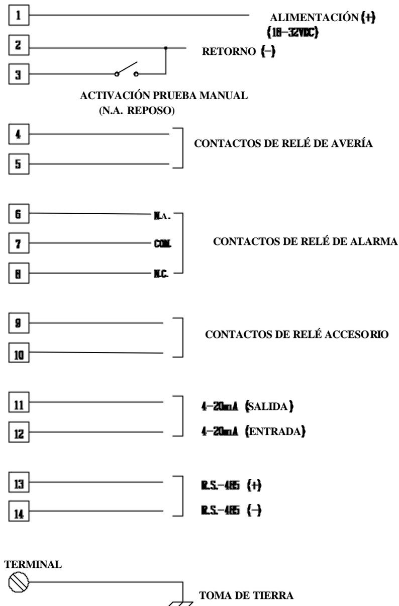
FIGURA 12: DIAGRAMA DE CONEXIONADO DEL DETECTOR DE LLAMA
