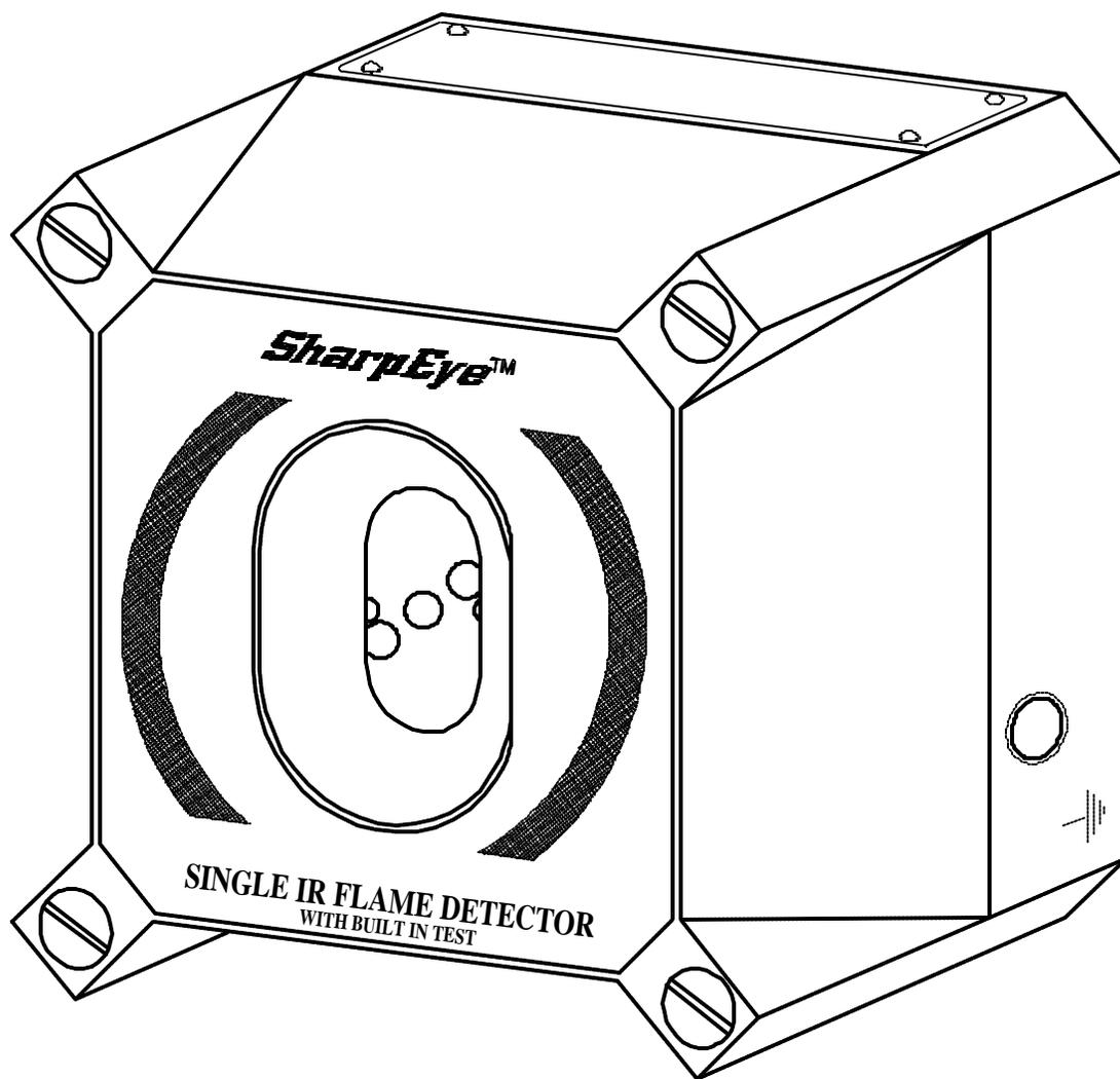
**FIGURA 1: DETECTOR DE LLAMA IR<sup>1</sup>**
