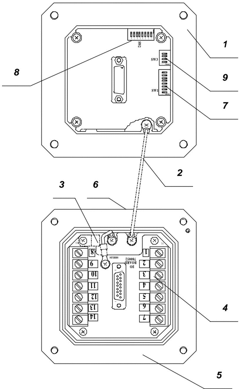
**FIGURA 11: DETECTOR DE LLAMA IR<sup>3</sup> SIN TAPA**
