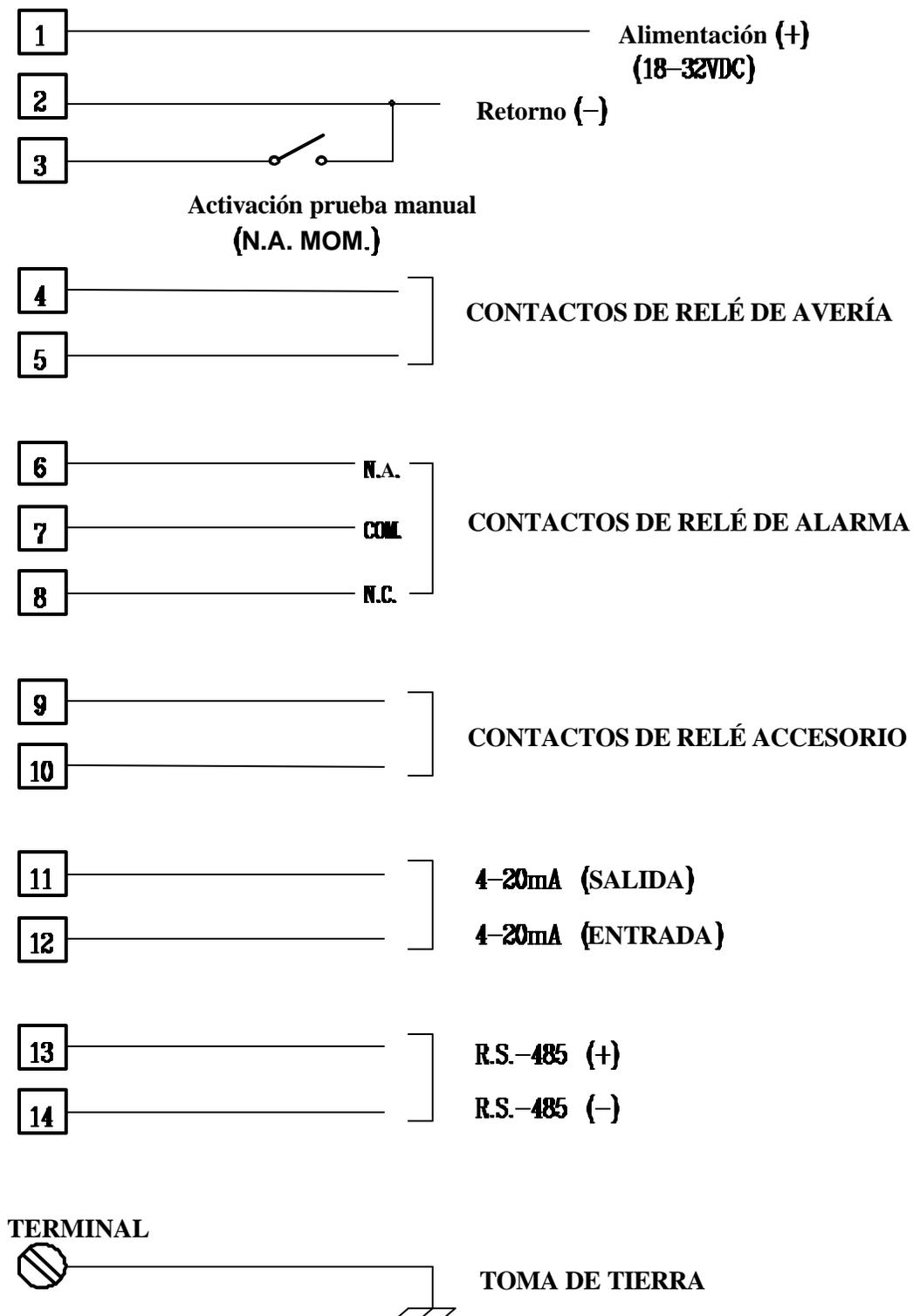
**FIGURA 10: MONTAJE DEL DETECTOR DE LLAMA - DIAGRAMA DE CONEXIONADO**
