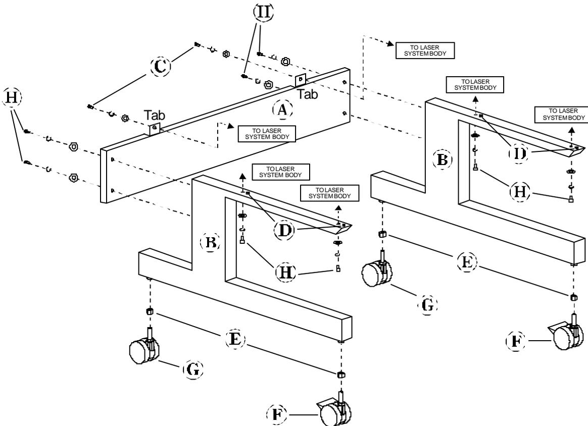
1. Attach the back panel (A) to the legs (B) with the 4 screws and lockwashers (C).
