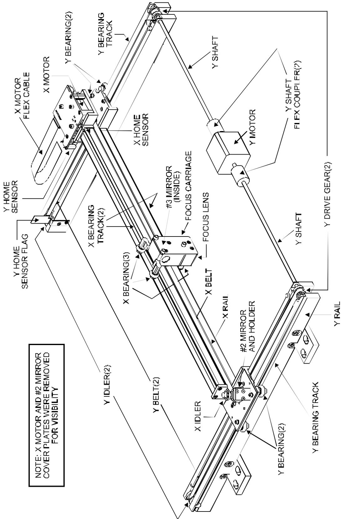
NOTE: X MOTOR AND #2 MIRROR COVER PLATES WERE REMOVED FOR VISIBILITY
