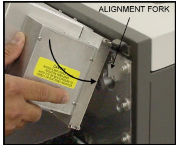
Pick up the Laser Cartridge by the sides. Tilt the Laser Cartridge downward on a 30-degree angle. Mount the cartridge onto the Mounting Blocks by placing the upper “V” groove of the cartridge on top of the Mounting Blocks. Slide the cartridge to the right until the Alignment Plate of the Laser Cartridge makes contact with the inside of the large plate of the Alignment Fork and is centered in the gap in the Alignment Fork between the small and large plates of the Alignment Fork.
