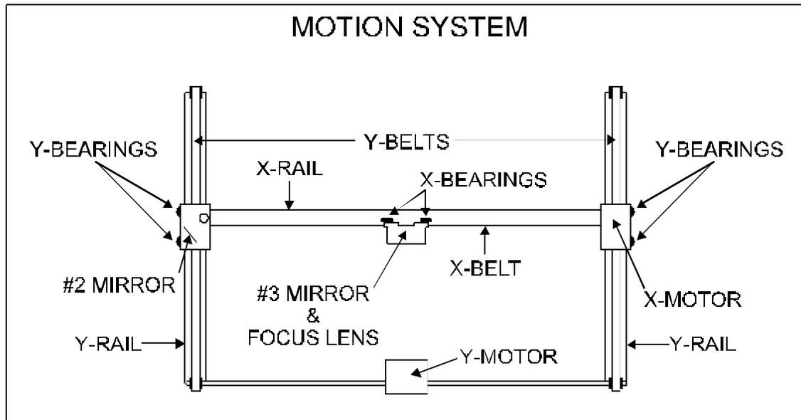
The CPU controls the movement of the motors, which moves the mirrors and focus lens across the engraving area and over the material. At the same time, it is synchronizing the laser pulses with the position of the focus lens. It is this precise positioning and timing of the laser pulses that produces the highest quality and fastest speed of engraving.
