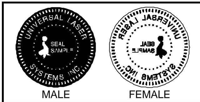
The laser system can be used to make dies for seal presses. It can engrave and cut out a typical Notary Seal in less than 5 minutes. Create the male with a white graphic and a black background. Mirror the image and invert it by making the background white and the graphic black. Add a .010 inch black outline to the graphic portion of the female side. This will give the greater clearance to the female side to prevent the paper from piercing through when the male side of the
