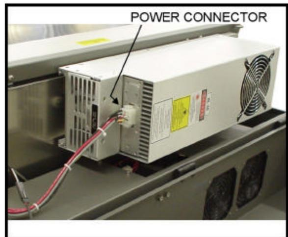
Plug in the Power Connector. The connector is keyed so it will only insert one way.
