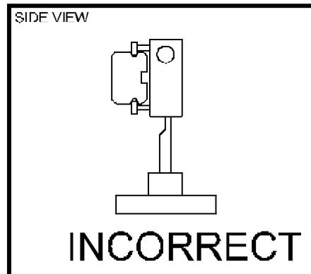
**WARNING:** Be careful not to position the tool underneath the focus lens as this can damage the lens if the table is driven up into it.
