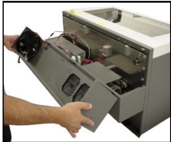
Gently fold back the rear cover. Visually locate the two Mounting Blocks, the Laser Latch, Alignment Fork, and Power Connector. Notice that the Alignment Fork has two plates, one small and one large. Locate the gap between the two plates.
