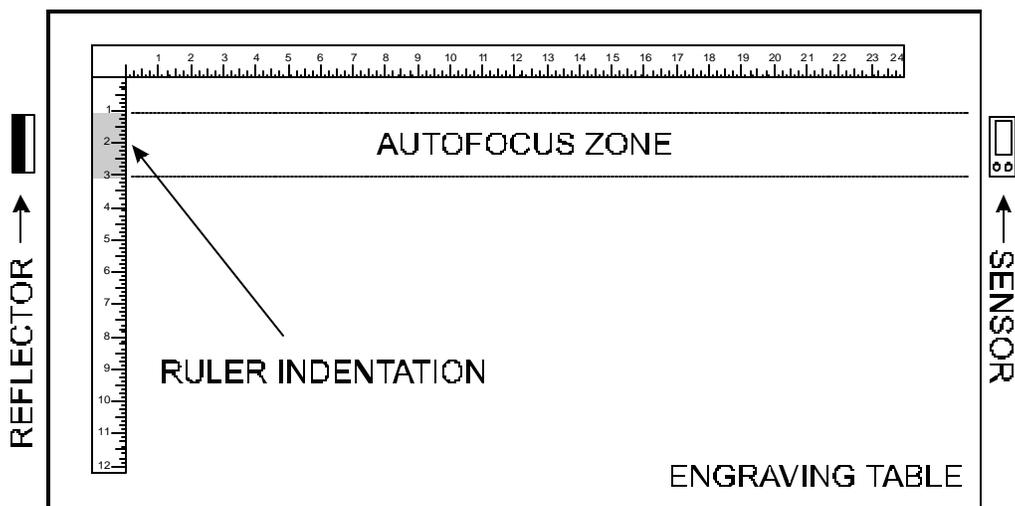
To clean these parts, dampen a soft cotton cloth with water and gently wipe across the reflective surface in one direction. **DO NOT** rub hard or create scratches in the plastic, otherwise the AUTOFOCUS system will malfunction. **DO NOT** use any type of cleaners, only use water or a light solution of hand soap and water on the sensor or reflector.
