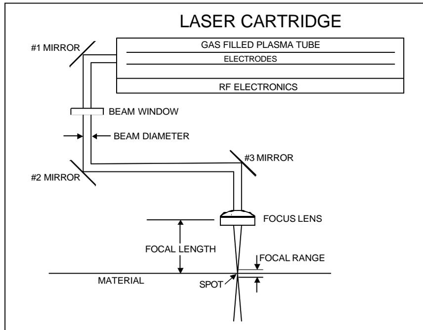
The laser cartridge receives power from the 48VDC power supply and its "trigger signal" from the CPU. When the laser system is powered on and the trigger signal comes from the CPU, the RF electronics produce a high frequency AC signal across the electrodes located inside the plasma tube. This causes spontaneous photon emissions from the gas mixture that produces an invisible, infrared light beam at a frequency of 10.6 microns.
