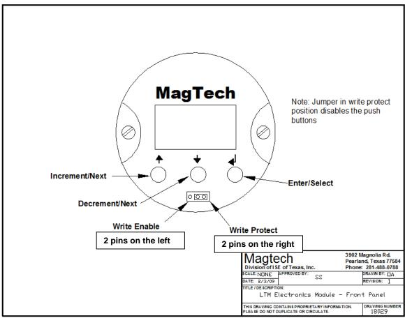
Figure 15. Front Panel of Electronics Module
