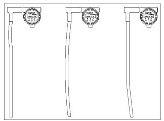
Figure 8. All damaged sensor probes
