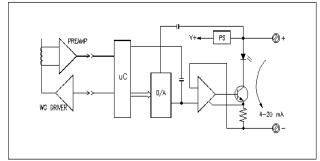
Figure 7. Basic Transmitter Block Diagram
