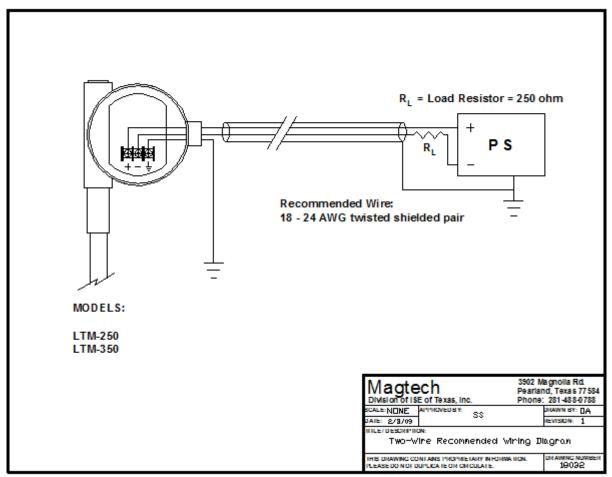
Figure 13. Recommended Loop Wiring
