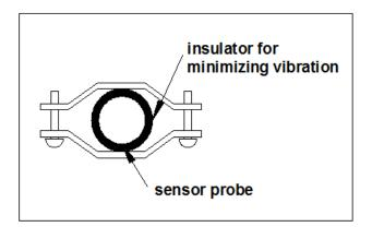
Figure 11. Insulator for high vibration
