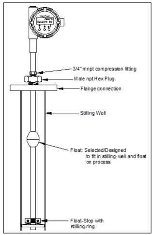
Figure 4. Transmitter with a Stilling-well
