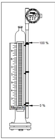
Figure 2. Gage mounted transmitter
