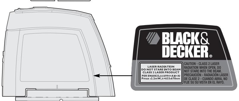
Avoid exposure-Laser radiation emitted from this aperture.
