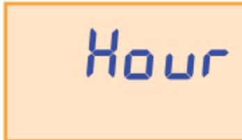
Pressing the «▲» and «▼» keys for 3 seconds allows you to program the parameters for the hour, minutes, year, date, month, height above sea level of the Meteorological Station and the screen luminosity function.
