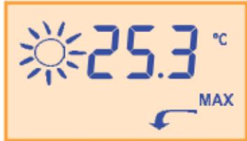
The screen shows the maximum temperature since the last start-up. Press «▼» to delete the maximum and minimum.
