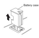
4 Slide the battery case back into the battery holder and press firmly so that the battery case locks into place.
