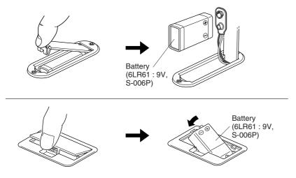
\* When changing batteries, pay close attention to the +/- polarity markings as shown in the illustration above.
