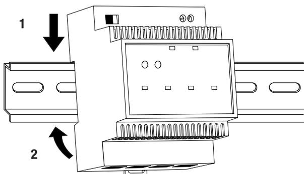
Make sure that the device is well fixed on the DIN rail.
