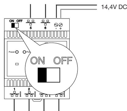
LAN port 1-4 (PoL enabled), Ethernet connections for:
