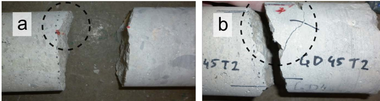
Fig. 47 - Atypical failure: (a) stone chip protruding on one side, (b) on two planes.
