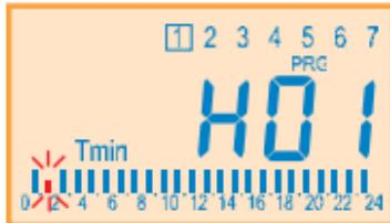
If the **Tmax**, **Tmin** or **Freeze** protection selections should remain the same, continue to confirm by pressing «OK». In order to change any of the selections, press «SELECT».
