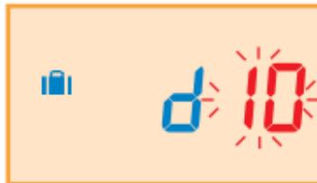
The screen displays the **TRAVEL** mode and the period of time flashing.
