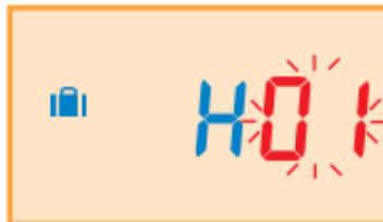
By pressing and holding the «OK» button for five seconds (only from **AUTO** or **MANUAL**), the **TRAVEL** mode is entered (Timed Off for holidays).
