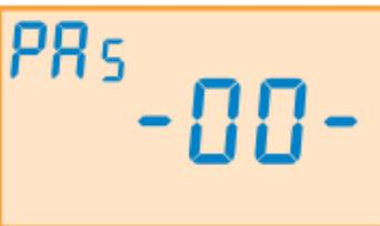
In order to access the Installer Settings programming, press the «▲» and «▼» buttons for more than 5 seconds.
