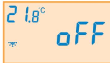
By pressing and holding the «MENU» button for five seconds (only from AUTO or MANUAL), the DISCONNECT mode is entered.
