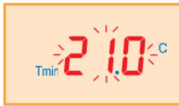
The current **Tmin** temperature is displayed flashing on the screen.
