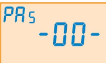
When the Installer Settings are accessed again, the password is requested. The screen is configured as follows:
