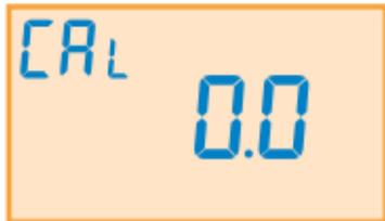
**CAL** → Temperature sensor calibration (offset).
