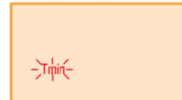
Press the «MENU» button until **Tmin** is displayed flashing on the screen.
