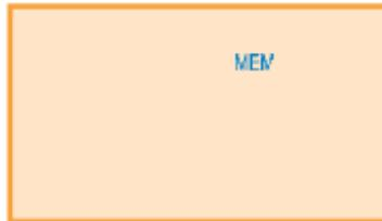
By pressing the «OK» button after programming the Installer Settings, the programmed data are automatically recorded, thereby indicating **MEM** on the screen.
