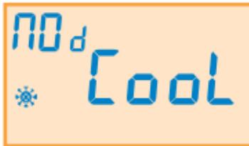
**Mod** → Type of control: Heating or Air Conditioning.
