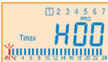
In order to select between **Tmax** and **Tmin** or **Freeze protection**, press the «SELECT» button.
