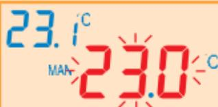
The temperature is displayed flashing on the screen (with the value below the ambient temperature).
