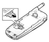
4. Insert the SIM card under the two tabs, ensuring that the cut corner is lower right and the gold contacts of the card face into the phone.
