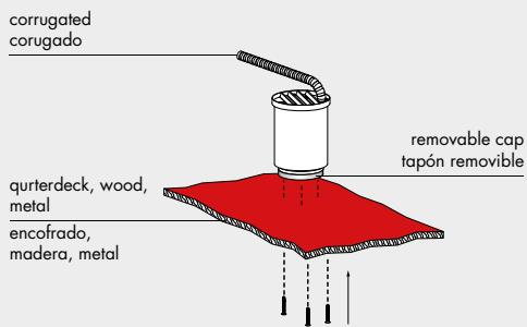
install the light fitting, providing a removable recessed stopper appropriate for the depth required. secure the formwork with screws.
