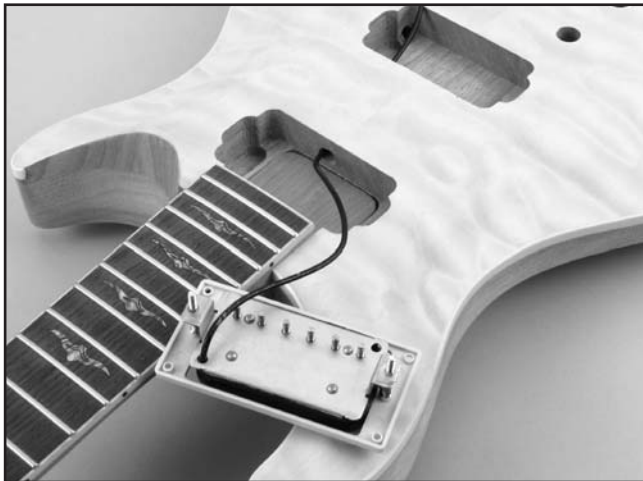
Figure 17. Neck pickup wire.
