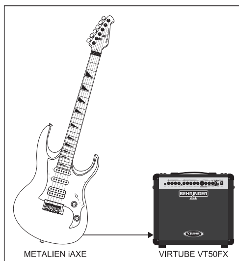
Fig. 4.2: Connection to a guitar amp
