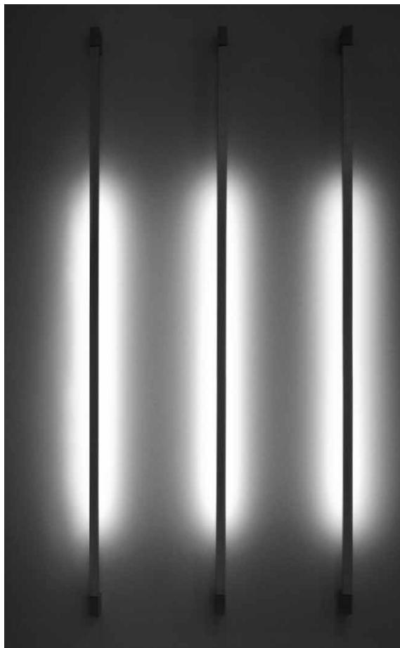
modular light system for interiors in matt silver oxidized extruded aluminium. available for walls or ceiling mounting. it can be fitted with 35W, 28W and 21W, 120V T5 fluorescent tubes with an overall length of the light fitting equal to 84.31", 68.50", 56.69". the power supply unit is located at one end of the electrified module. the fluorescent tube fitting can rotate 350° on the wall attachments on a vertical axis. it has been designed also as a modular system in a chain.
