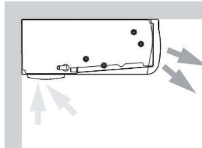
VENTILADOR-CONVECTOR A EMPOTRAR FC INSTALADO HORIZONTAL (EN FALSO TECHO)
