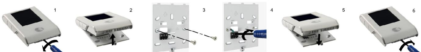
**EN** Note: A cross-head type screwdriver is required during installation process
