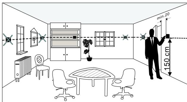
**EN** The room thermostat should be mounted in a location where the air temperature can be measured as accurately as possible without getting adversely affected by direct solar radiation or other heat or refrigeration sources.
