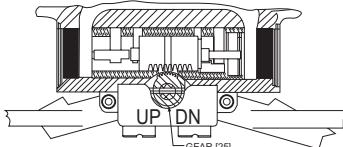
STEP 3 :- ASSEMBLE O-RINGS [16] TO VALVES [17] AND [19] AND ASSEMBLE VALVES INTO HEAD AS SHOWN. ASSEMBLE O-RINGS [18] TO ADAPTERS [29] AND O-RINGS [20] TO VALVE CAPS [21] AND ASSEMBLE TO HEAD.
