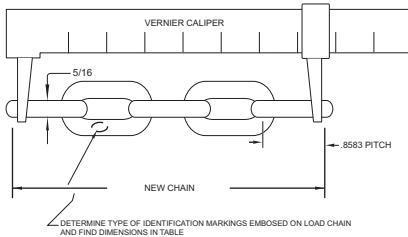
IT IS NOT INFERRED that a chain is safe prior to the occurrence of elongation of the chain. It is inferred ONLY, that when said elongation is evident, the chain must be replaced. Other factors, such as those mentioned as a visual check, may render chain unsafe long before replacement due to elongation is necessary. NOTE: New chain should never be used on a worn pocketwheel, replace chain and pocketwheel as a pair. Chain should also be replaced when replacing brake shoes.
