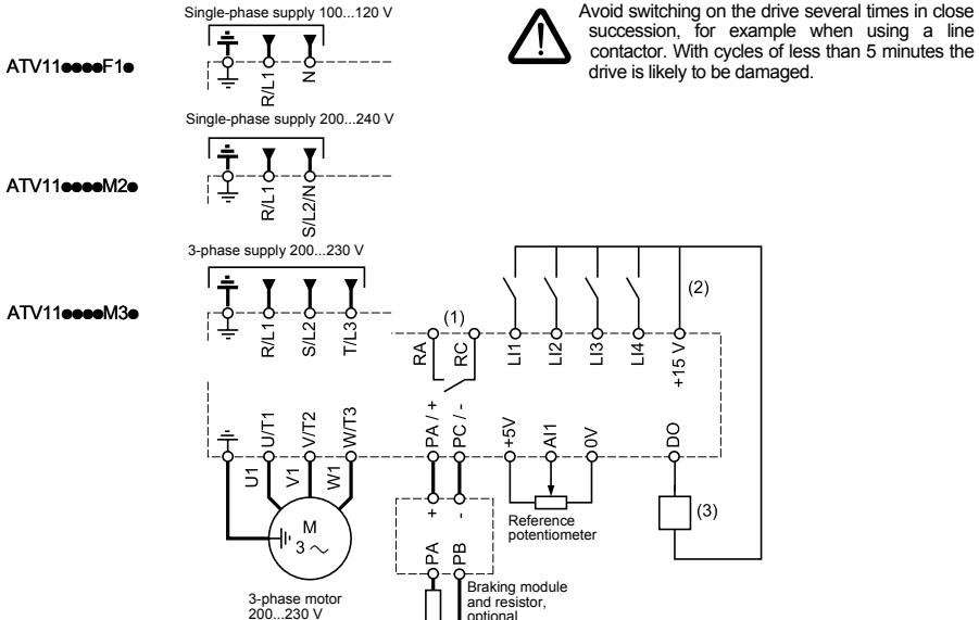
(1) Fault relay contacts, for remote indication of the drive status.
