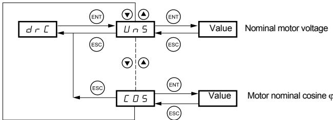
The parameters in clear boxes can only be modified when the drive is stopped and locked.
