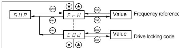
When the drive is running, the value displayed is that of one of the monitoring parameters. The default value which is displayed is the motor reference (parameter FrH).
